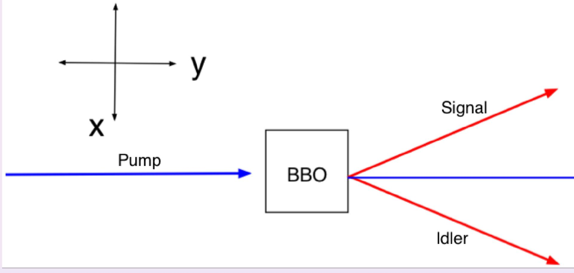
Inside a type-II beta Barium Borate crystal, photons of wavelength approximately equal to 400nm are spontaneously down-converted into pairs of infrared photons. Each pump photon is converted into a signal and idler photon, which together conserve the momentum and energy of the pump.
