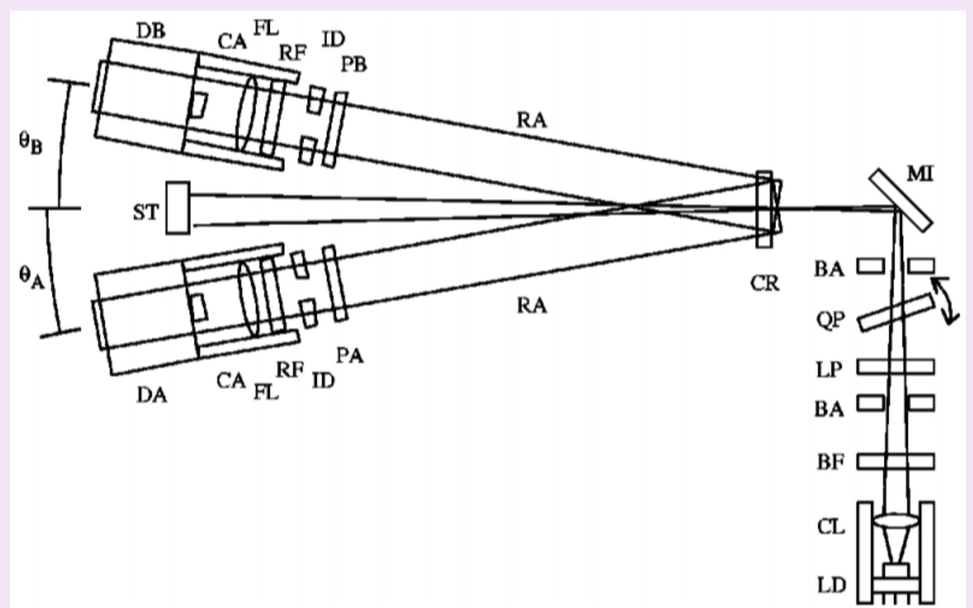
Light from a commercial diode laser,  $\lambda = 404\text{nm}$ , passes through a BBO crystal where it is down-converted into cones of infrared light. The intersections of these cones is picked out by the height of the detectors, and we sweep through angles in an attempt to maximize the observed count rates. We are interested primarily in the degenerate case.
