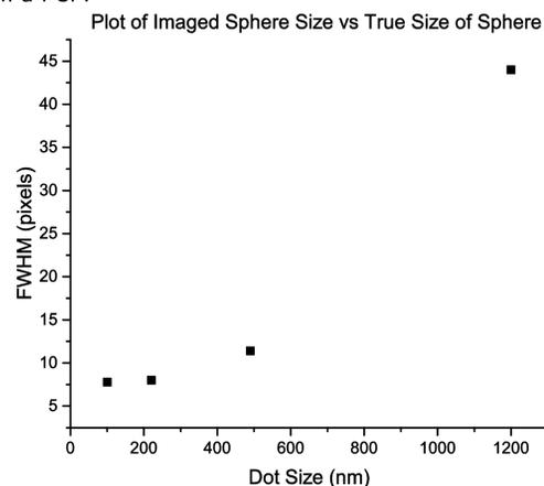
This allows us to see that as we expected, the measured width of the calibration spheres decreases linearly up until a sphere size of around 250nm. Therefore, this is roughly the diffraction limit of our microscope in the transverse imaging mode, and so this is the imaging limit which we hope to overcome through deconvolution.
