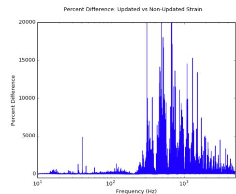
We can see that the greatest difference in the updated versus the non-updated strain occurs at higher frequencies. This is to be expected, since the correction made in the cavity pole filter update has the most effect on high frequency signals.
