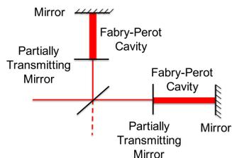
LIGO loses sensitivity to gravitational waves at frequencies higher than the frequency of the inverse of the light storage time in the Fabry-Perot Cavity ( $f_c$ ). The purpose of the Fabry-Perot filter is to model the decrease in sensitivity that the detector has to frequencies above this threshold. The Fabry-Perot filter is a low pass filter in the frequency domain which is used to filter out signals from the data with frequencies higher than that of the Fabry-Perot Cavity ( $f_c$ ).
