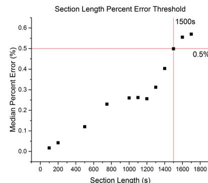
From this graph it was determined that the Fabry-Perot filter should be updated every 20 minutes which corresponds to every 1200 seconds. This value was shown to be safely below the 0.5% median error threshold.
