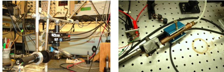
We built the prism coupler system shown at the left using two suspended Newport rotating stages and photomultiplier tube (PMT) operated by LabView. The image at the right is the prism with the pneumatically operated coupling plunger which applies 30-40 psi to the back of the sample onto the back of the prism
