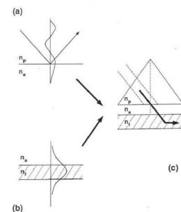
Fig. 4 Optical tunneling in a waveguide PCT<sup>4</sup>
