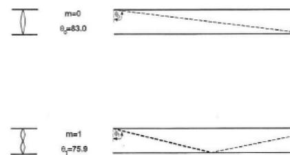
Fig. 5 The supported modes in a thin film<sup>4</sup>
