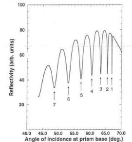
Fig. 7 The spectrum of a 1.400  $\mu\text{m}$   $Zn_{0.725}Cd_{0.275}Se$  thin film with a 632.8 nm HeNe laser from Peiris's work<sup>4</sup>.
