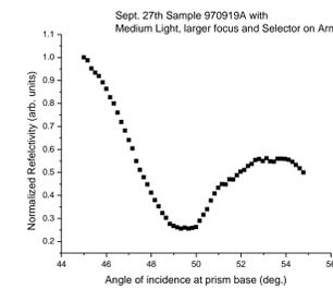
Fig. 6 The first observed dip in a 2.300  $\mu\text{m}$   $Zn_{0.91}Cd_{0.09}Se$  thin film with 488 nm HeNe laser. Subsequent dips were difficult to observe.
