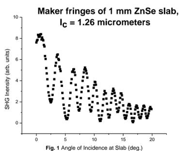
Fig. 1 The interference patterns from the Maker fringes can easily be seen with a bulk slab
