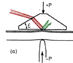
Fig. 8 Localized pressure causing deformation of the film<sup>3</sup>.
