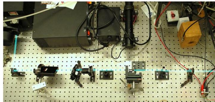
488 nm light passing through an iris, Fresnel rhomb, optical density filter, polarizer, spatial filter, + 6 inch lens, and an iris into the PCT system.
