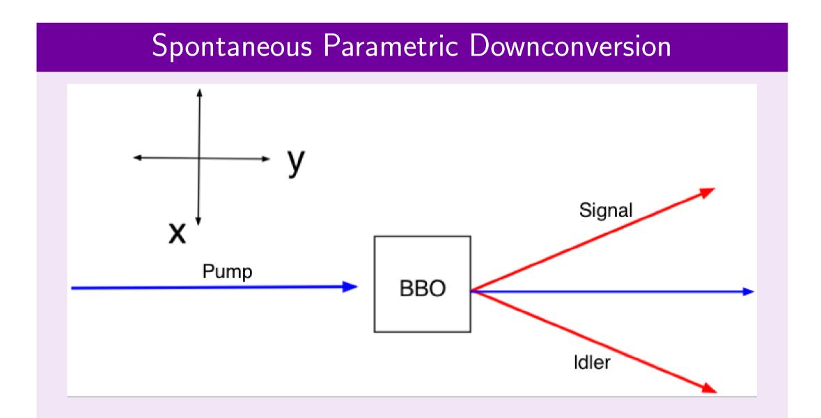
Inside a type-II beta Barium Borate crystal, photons of wavelength approximately equal to 400nm are spontaneously down-converted into pairs of infrared photons. Each pump photon is converted into a signal and idler photon, which together conserve the momentum and energy of the pump.
