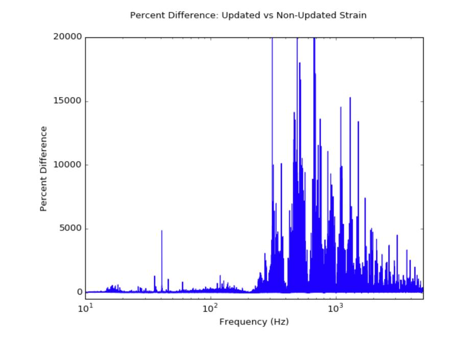
We can see that the greatest difference in the updated versus the nonupdated strain occurs at higher frequencies. This is to be expected, since the correction made in the cavity pole filter update has the most effect on high frequency signals.
