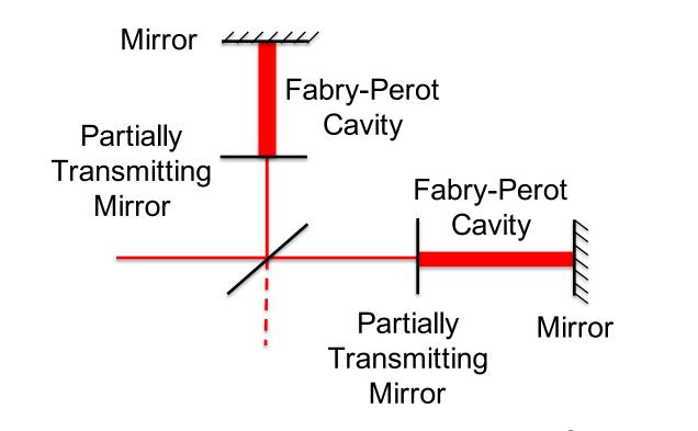
LIGO loses sensitivity to gravitational waves at frequencies higher than the frequency of the inverse of the light storage time in the Fabry-Perot Cavity ( $f_c$ ). The purpose of the Fabry-Perot filter is to model the decrease in sensitivity that the detector has to frequencies above this threshold. The Fabry-Perot filter is a low pass filter in the frequency domain which is used to filter out signals from the data with frequencies higher than that of the Fabry-Perot Cavity ( $f_c$ ).
