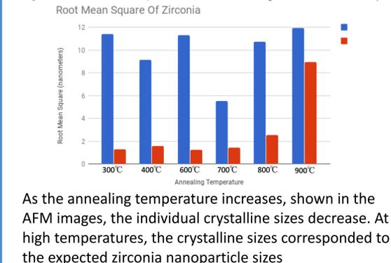
As the annealing temperature increases, shown in the AFM images, the individual crystalline sizes decrease. At high temperatures, the crystalline sizes corresponded to the expected zirconia nanoparticle sizes
